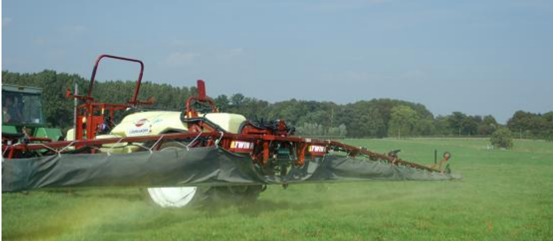
Figure 5.2: Hardy Commander Twin Force trailed field sprayer with 27 m boom, Twin air assistance and a tank volume of 3200 litres
