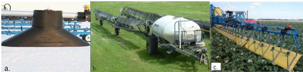
Figure 2.7: Different types of shielded sprayer booms: (a) WindCone (Brandt Industries, Ltd.) (b) Flexicoil (Ag Shield Mfg) (c) Släpduk (Viby Teknik)
