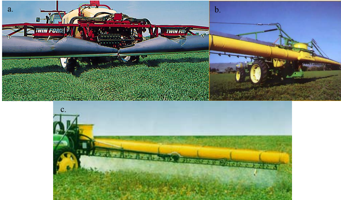
Figure 2.5: Some air-assisted sprayers (a) Hardi Twin (b) Degania (c) Spray-Air
